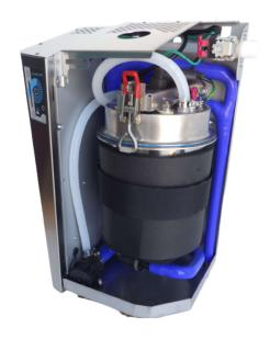
**steamOres** (RES) residential humidifier by **steamOvap**® is an electric steam generator that uses water immersed resistive heating elements to produce pure and sterile steam to humidify your home or office during winter.
