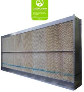
**AEM** evaporative humidifier and cooler using evaporative media is designed to be installed in Air Handling Unit (AHU) or ventilation duct. Water is circulated in the evaporative media, as hot air is passing through the wet media, water is evaporated by the latent energy of the air. As a result the air gets cooled off up to 12°C and humidified at the same time.
