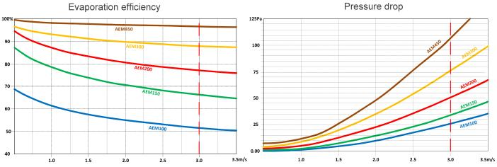
Note: Installation of droplet separator is required when air velocity is above 3.0m/s
