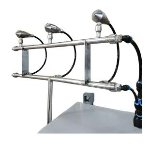
ACA dry fog atomizer are supplied with water and compressed air. Atomizer's **patented** acceleration chamber creates an airflow pattern reaching supersonic speeds. The airflow sucks in water from a venturi column. The impact between the supersonic flow of air and the water generates shock waves, which produce the micro-droplets. The "solid con" jet of micro droplets forms a uniform "dry fog" which evaporates quickly into the air.
