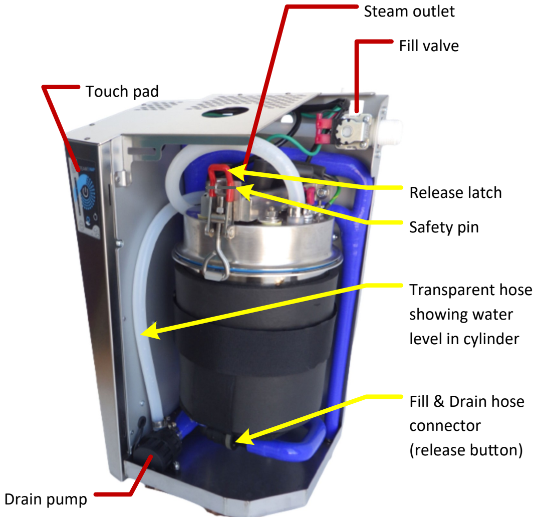
Figure 19 – RES steam cylinder and key components
