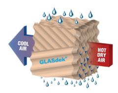
AEM, Evaporative humidifier and cooler using media is designed to be installed in Air Handling Unit (AHU) or ventilation duct. Water is circulated in the evaporative media, as hot air is passing through the wet media, water is evaporated by the latent energy of the air. As a result the air gets cooled off up to 21°F [12°C] and humidified at the same time.
